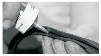
5. Apply weather stripping adhesive in several places within the groove on the cowl vent seal. This will hold the seal into place during reassembly.
