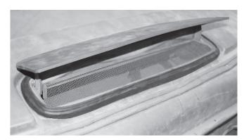
8. Reinstall the 8 vent mechanism screws then reattach the cowl vent door.
