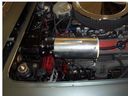
Connect the black wire with installed ring terminal to engine ground.
