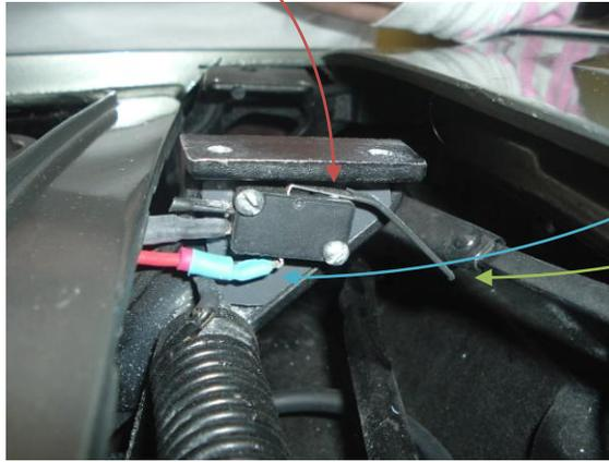
Make sure the wiper arm is completely in home position when adjusting the micro switch.
