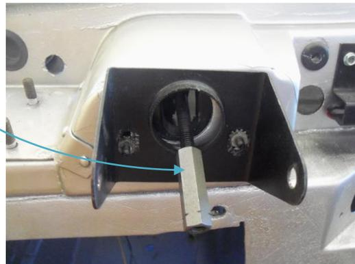
Now file the Aluminum bracket on the left, right and bottom of the opening a 1/8" to give room for the actuator piston to move.
