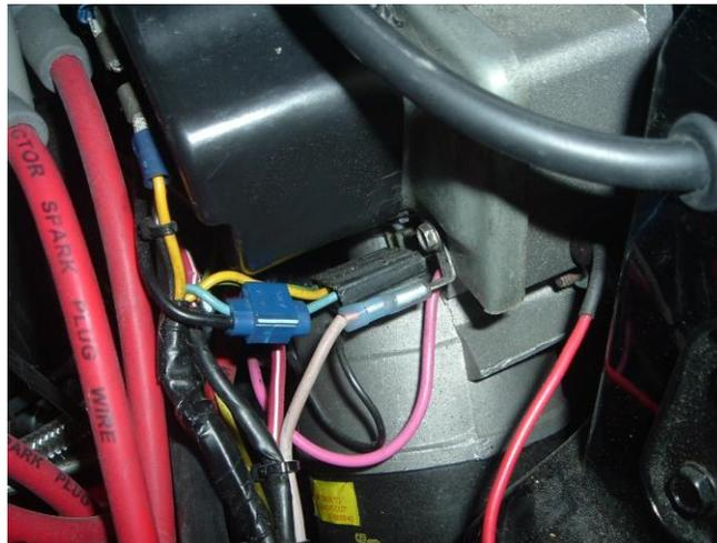
Up to early 69 models switch the green wire to ground when the wiper switch is activated. To check for the correct wire, connect a test light to the positive terminal on the alternator and to the blue wire if it lights up when you turn the wiper switch on you have the correct wire. If not, check the green wire.
